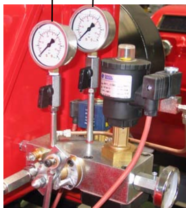
Fig. 32 - Oil pressure governor
