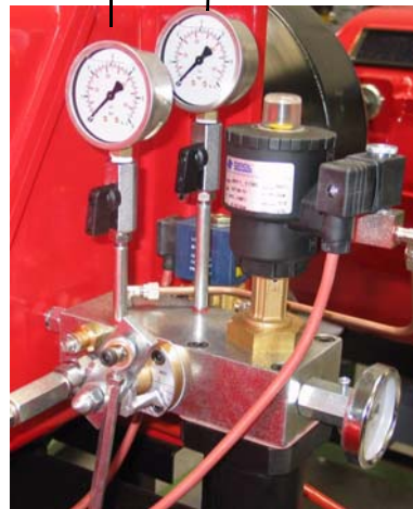
Fig. 25 - Oil pressure governor
